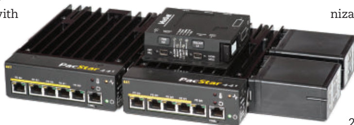
PacStar 400-series small communications modules enable engineers to customize systems.
