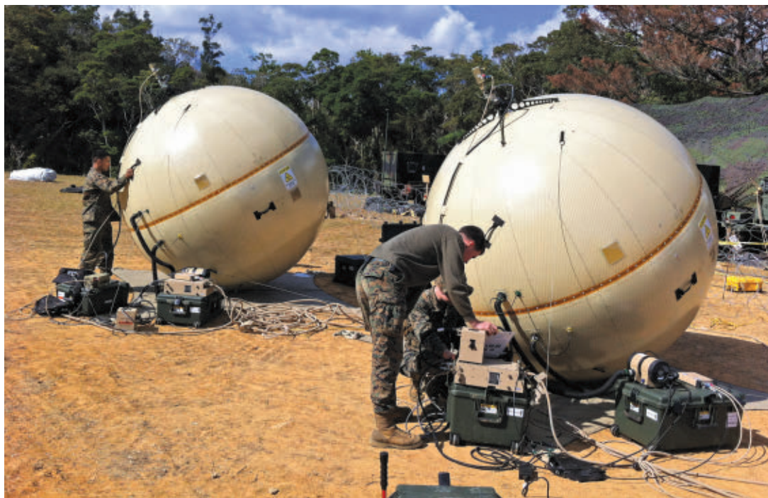
GATR, a business within Cubic Mission Solutions, provides inflatable satellite communication (SATCOM) antenna solutions designed to offer portability, low cost of ownership, reliability in extreme environments, and ease of setup.
