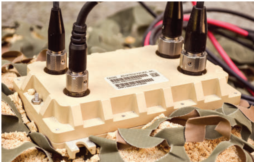
Advtech Pacific’s Tactical Cross-Domain Solution (TACDS) automatically performs deep content inspections on information moving across classified and unclassified domains.
